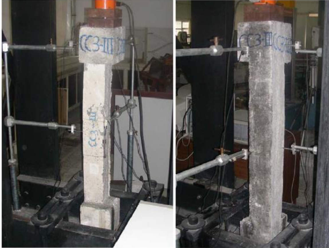
Fig. 4. (a,b) The typical failure mode of the column specimens.
